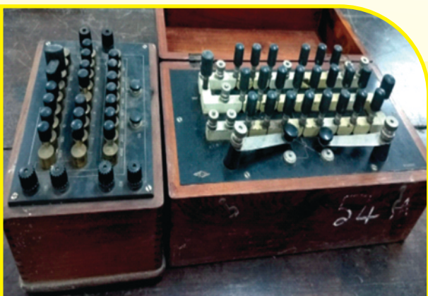
Earlier Form of Wheatstone network to find the unknown resistance (Post Office Box)
