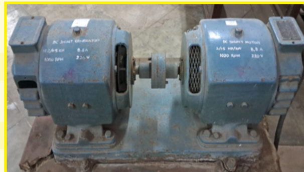
Hopkinson Testing set 2 HP DC machines (1935)
