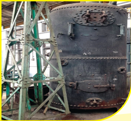
Vertical Steam Boiler made in England
