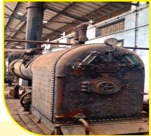
Horizontal Steam Boiler made in Madras
